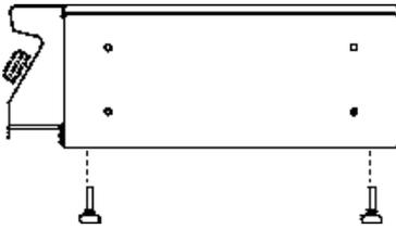
**DO NOT USE THE BARBECUE IN THE TOP VERSION WITHOUT FITTING THE FOOT FIRST.** Place the top on a flat surface and ensure it is stable by tightening the foot adjustment screws.
