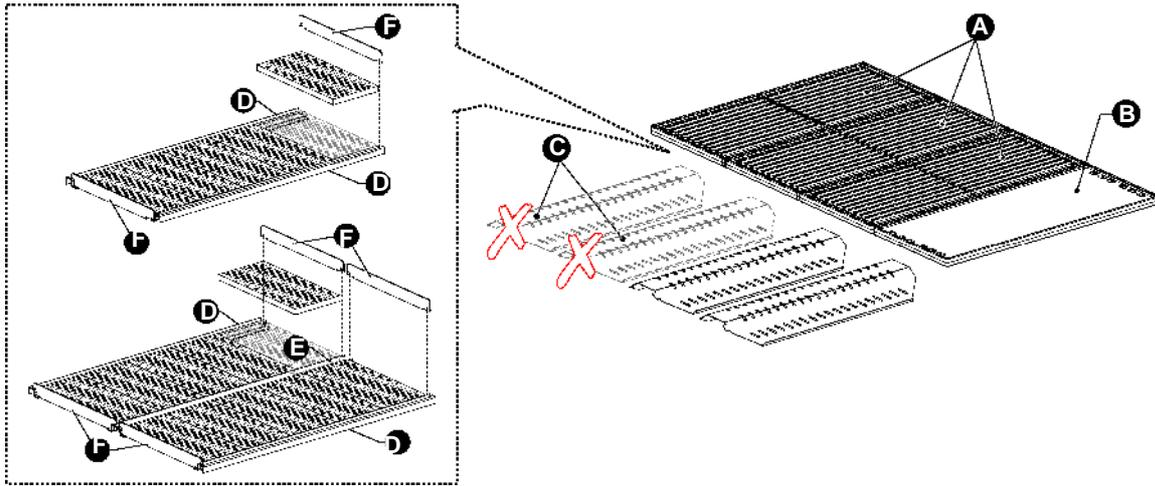
1. Remove the grill grates "A", griddles "B" and disperser "C" (one per kit to be installed).
